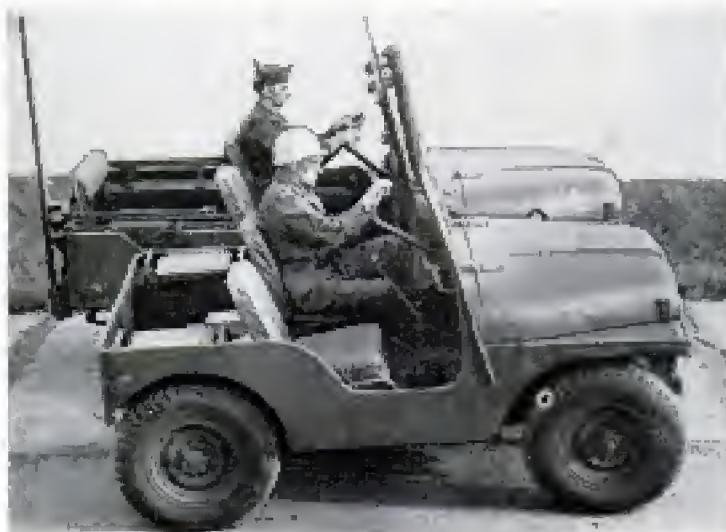
←Aero Jeep, although three feet shorter than older Jeep, can also carry four men
